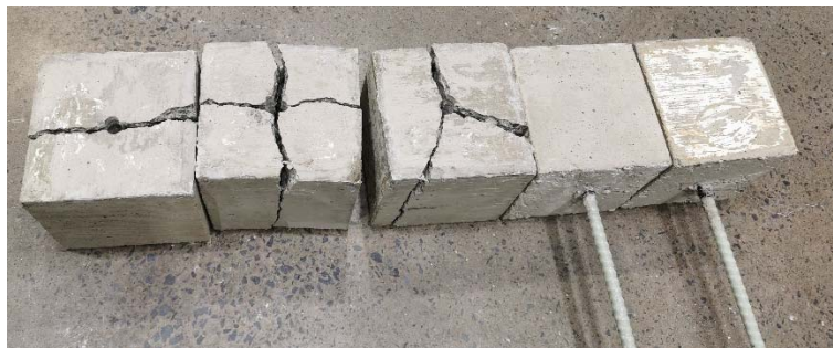
Figure 4: The failure mode of the 15 mm (#5) MST-BAR® GFRP rebar.
