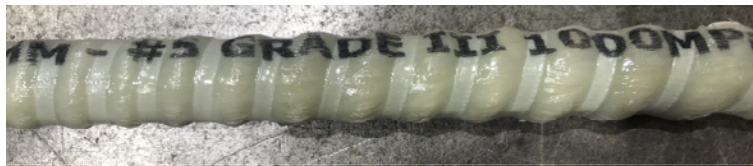
Figure 1: 15 mm (#5) MST-BAR ® GFRP rebar.
