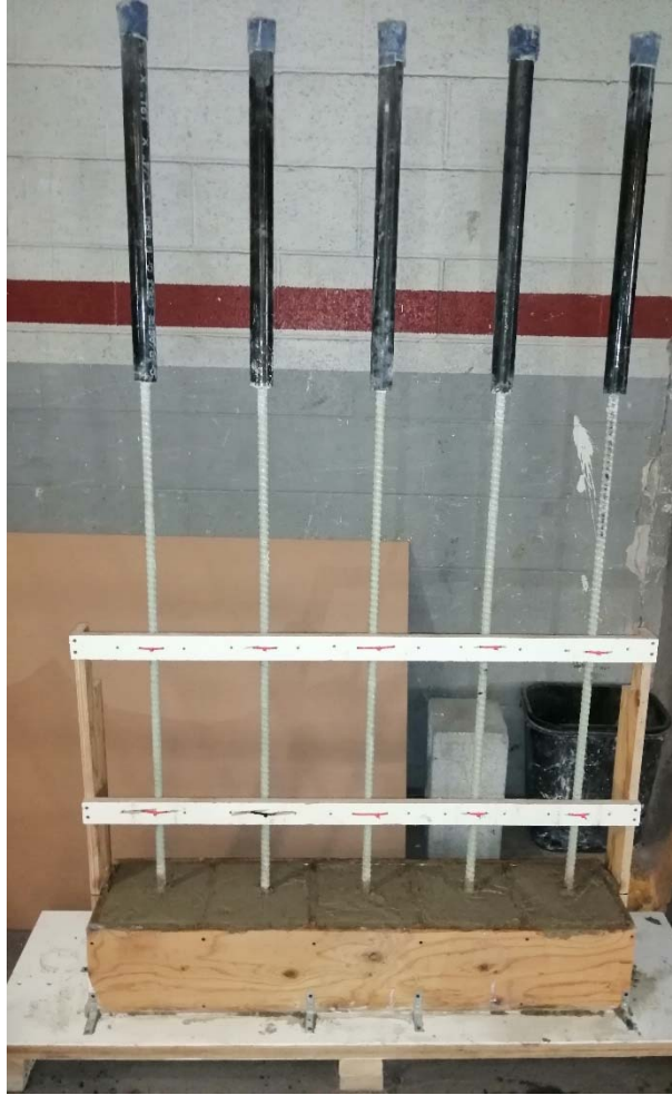
Figure 2: 15 mm (#5) MST-BAR GFRP rebars samples after the concrete pour.
