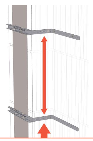
IMPORTANT NOTE: The Buck Brace shall be installed no less than 2 feet apart on a 6-inch core ICF Block and 18 inches apart on an 8-inch core ICF block. This minimum distance between braces will ensure adequate window and door opening bracing.
